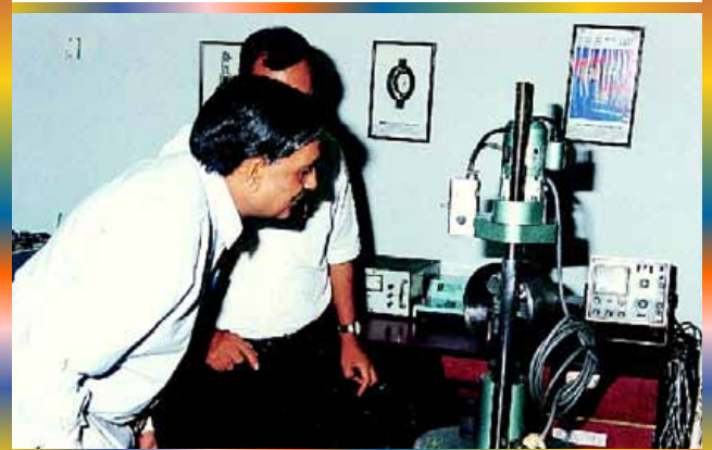
Dr. Kota Harinarayana, Director, Aeronautical Development Establishment, Bangalore is looking at the functioning of 5000 KGF Morehouse Universal Calibrating Machine and Proving Ring (accuracy : 0.0125%) at Vaiseshika Metrology Laboratory.
