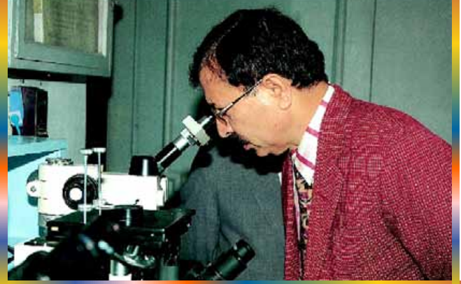
Dr. S. E. Hasnain observing a Metallographic specimen through Micro Hardness Tester at Vaiseshika Facility
