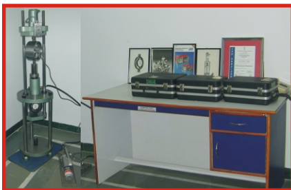
Ring Dynamometer under calibration on MOREHOUSE Universal Calibrating Machine
